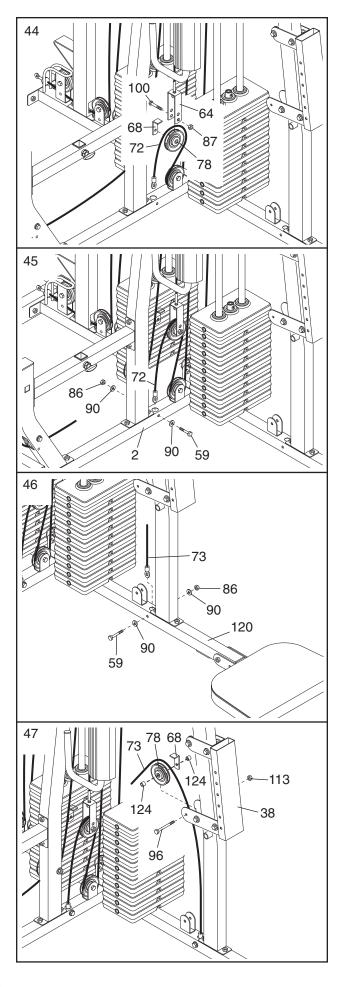
Wrap the Squat Cable (73) under a 3 1/2" Pulley (78). Attach the Pulley to the indicated bracket on the Long Base (120) with a 3/8" x 1 3/4" Bolt (93) and a 3/8" Nylon Locknut (87).
